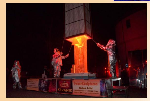
After overnight preheating aimed at completing the drying of the colossus, we started the firing itself at 5 am. I have piloted all sorts of gas-fired kilns in my life as a ceramist and this one did not frighten me more than another. No problem – even if it was necessary to climb a ladder to handle the opening of the chimney—it wasn't the first time!
